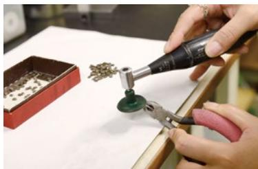
An inspection room set up on the second floor of the factory. High-accuracy parts must be within as much as  $\pm 0.025\text{mm}$ .
