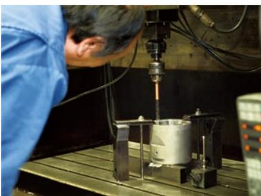
High technological capability is necessary to respond to special processing needs. All KHK die-sinking EDMs are made by Mitsubishi Electric, and the majority have been used for many years.
