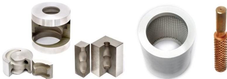
A processing sample. On the left is a sample of a helical hole drilled in a circular workpiece. Behind that is a sample of a spiral shape processed in a cylindrical workpiece interior. To the bottom right is a sample of a part where the processing entry point on the surface is narrow but widens internally. The second item from the right is a sample of several hemispherical patterns processed in a cylindrical workpiece’s interior. The far right shows the resulting electrode.
