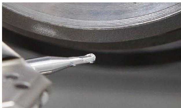
Cemented carbide end mills are manufactured by grinding cemented carbide alloy workpieces (part with pointed tip pictured in middle of photo) using a diamond grinding wheel (pictured above workpiece).
