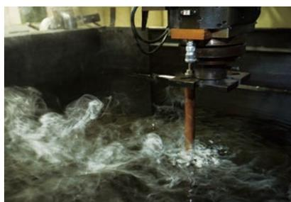
M85KC7 (left) – Mitsubishi Electric die-sinking EDM loaded with a giant workpiece measuring 1,350mm in diameter. The image on the right shows this part being processed.
