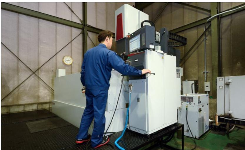
EA40M – Mitsubishi Electric die-sinking EDM introduced to KHK operations in January 2019. It is equipped with an extra-large processing chamber measuring 2200x1500mm.
