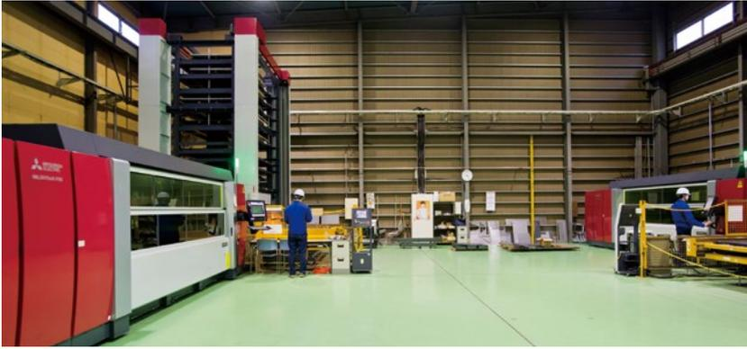
Tryan operates two ML3015eX-F60 machines. The fiber laser processing machine on the left is equipped with a 6-set sheet changer.
