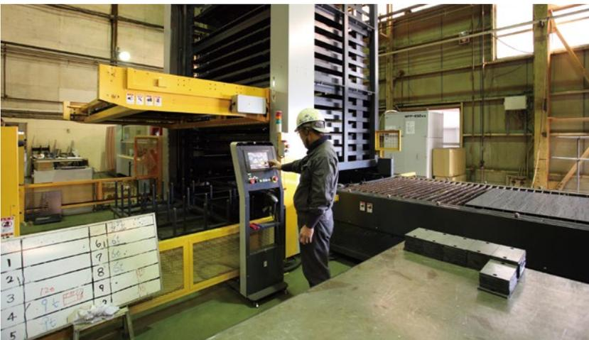
The 15-step stocker system introduced at the same time as the ML3015eX-F60. It automatically supplies sheet metal to the laser processing machine, and then automatically unloads the machine once processing is complete.
