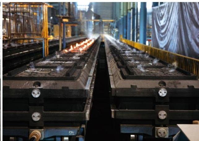
The Head Office Factory is responsible for casting. On the left is the pouring process and on the right is the cooling process. About 20% of the parts cast at the Head Office Factory are transported to the Kira Factory where they are processed with precision before being shipped.
