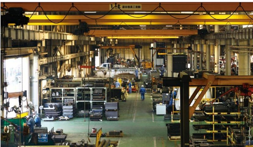
Simozato's head office and main factory is full of laser processing machines, machining centers, press brakes, welding robots, and CMMs.
