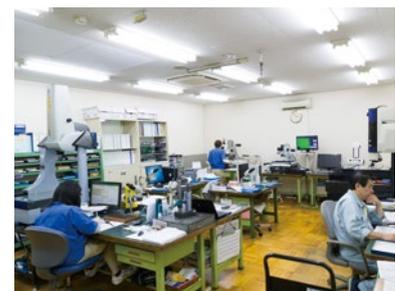
The "Inspection Room" contains various measurement devices, including a CMM and laser microscope.
