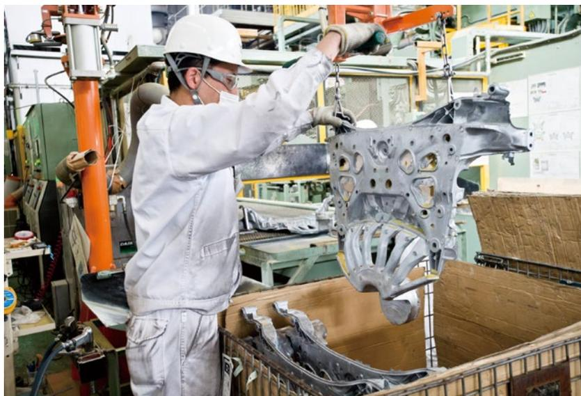
A hollow aluminum subframe made in a high-pressure die casting machine. After this, the part is machined on a turret center.
