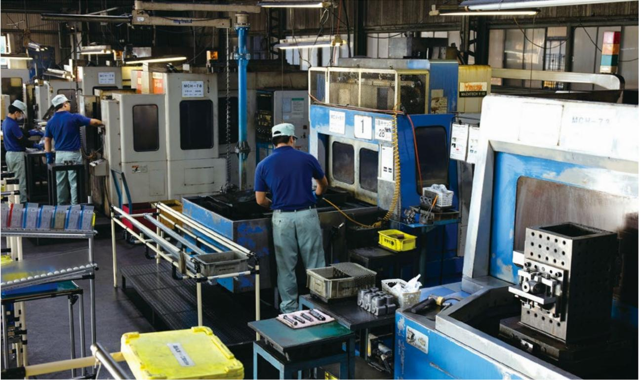
The Kira Factory of Nakanihon Casting has a line of lathes and machining centers. About 80 machine tools are in operation. About 30 of them are equipped with Mitsubishi Electric CNCs.
