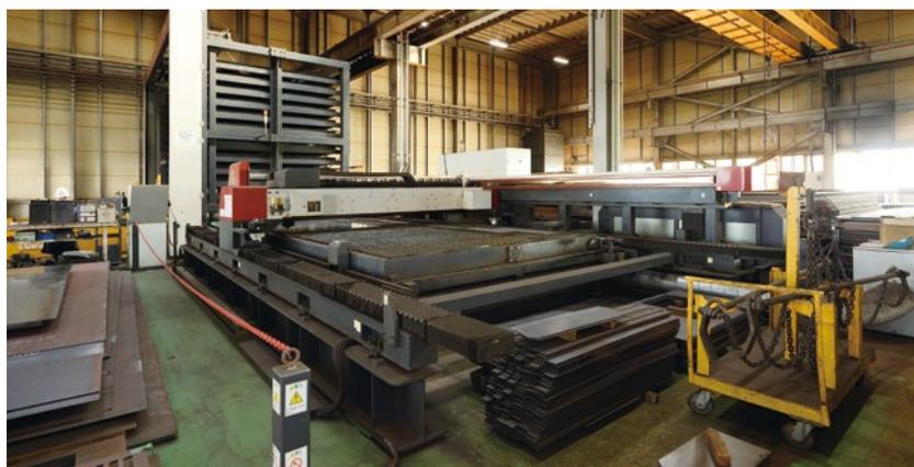
ML6030XL-45CF-R, a 4.5kW CO<sub>2</sub> laser processing machine capable of handling large steel plates up to 6100 x 3050mm. This machine is also equipped with a 12-step pallet changer.
