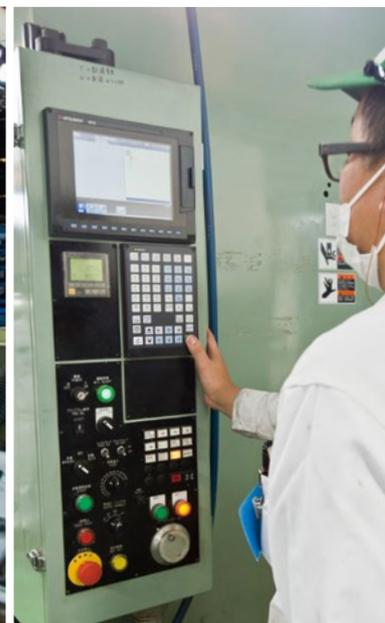
First Honda's BT#40 Turret Center combined processing machine is used for machining the hollow aluminum subframe. It is equipped with a Mitsubishi Electric M70 CNC.
