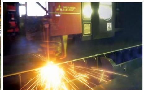
ML3015eX-F60, the 6kW fiber laser processing machine installed at Simozato in 2017. It features Japan's first twin tower-type pallet changer (10-steps + 12 steps).
