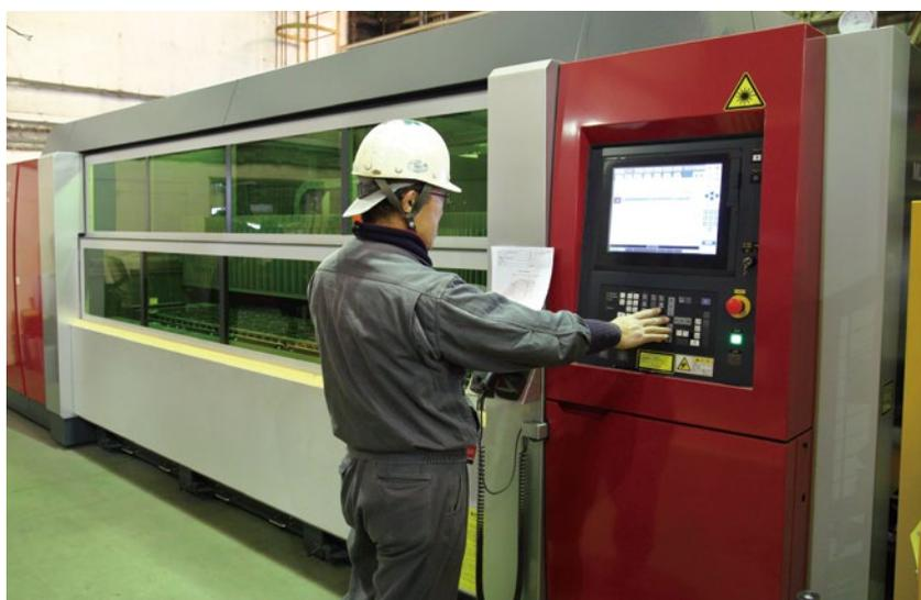
Mitsubishi Electric delivered a ML3015eX-F60 6kW fiber laser processing machine to Kasyu in March 2017. It features a zoom head that significantly reduces set-up changeover time.
