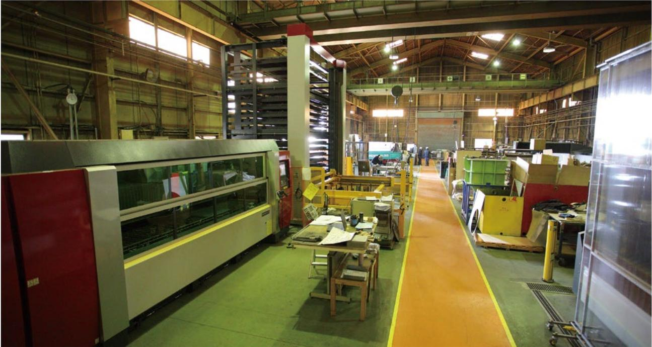
The NO.1 Company factory that oversees the processing of ferrous, non-ferrous, and non-metal materials. In addition to three laser processing machines, the company also owns a waterjet processing machine.
