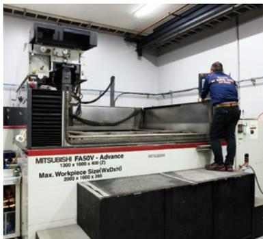
FA50V ADVANCE is a wire-cut EDM capable of processing extra-large workpieces with dimensions up to 2000 × 1600 × 395mm.
