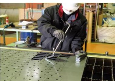
Removing a sheet metal workpiece that has been processed. The company processes sheet metal with thicknesses of 3.2-16mm in the ML3015eX-F60. It can also process material up to 25mm thick.
