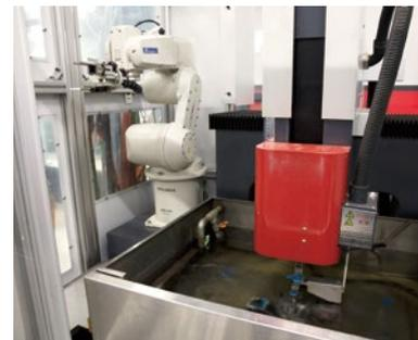
EMACH is a fine-hole drilling EDM equipped with a robot arm capable of automatically replacing electrodes. It can process fine holes as small as 0.2mm in diameter.
