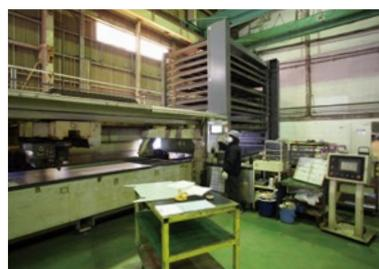
Mitsubishi Electric ML3015LZP, 3.5kW CO<sub>2</sub> laser processing machine introduced in 2001. Still actively being used 17 years later.
