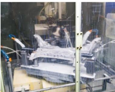
A hollow aluminum frame being machined in a turret center. This machine performs drilling, tapping, and milling.
