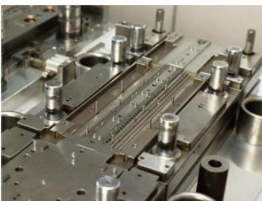
A sample of progressive dies for automotive parts. Nagumo's greatest defining feature is its high standard of processing accuracy.
