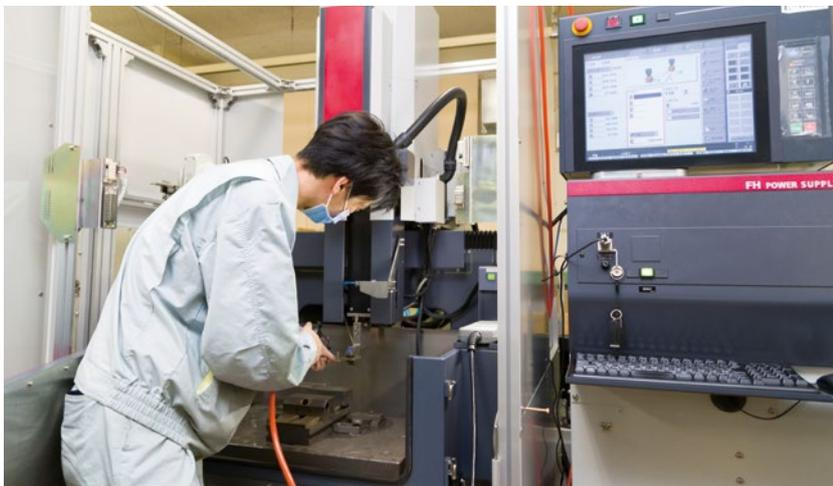
SH12 – Mitsubishi Electric’s fine-hole drilling EDM delivered to Nagumo in July 2018. Here, an operator is making adjustments prior to processing.
